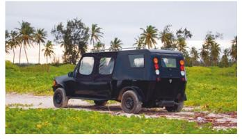
Four-wheel drive, a tough, tubular steel frame at an auto rickshaw price – the prototype Mobius One.
